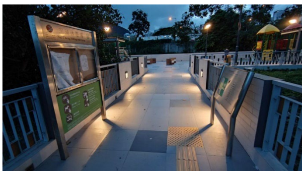
Sitting-out areas at the former Cat Street Bazaar site along Circular Pathway and Ladder Street in the Central and Western District (upper row) and at Nai Chung in the Tai Po District (lower row) with the use of paving units containing recycled glass, recycled timber benches, lightings with timer controls and light sensors.
