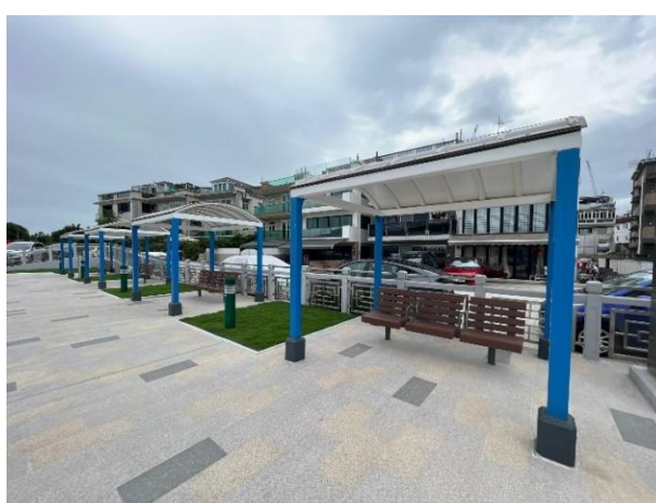
Sitting-out areas at Wah Lam Path (Extension) in the Southern District (upper row) and at Tseng Tau Village in the Tai Po District (lower row) with the use of paving units containing recycled glass, recycled timber plastic strip benches, lightings with timer controls and light sensors.
